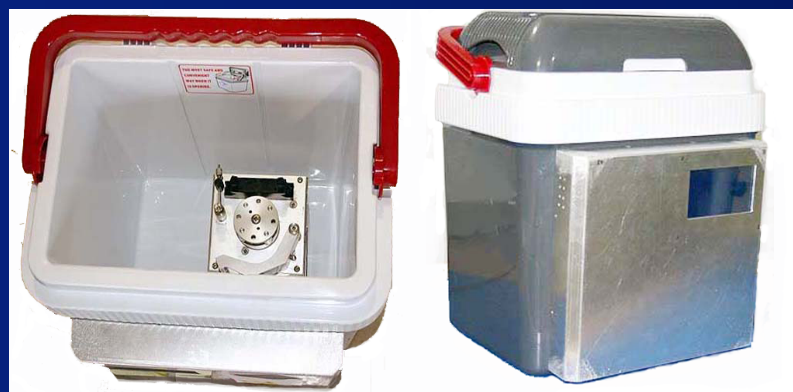
Figure 1: The Hibernicor Asporto heart preservation device consists of a lightweight pump, touchscreen microcontroller, and insulated thermo-electric cooler powered by 120 VAC or 12 VDC which maintains a temperature between 4.5 and 10 °C.
